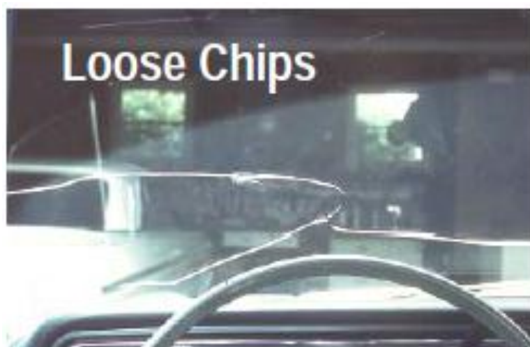
Figure 28: Windshield Damage Cause by Loose Chips (MTAG 2007)
