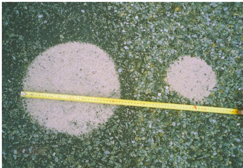
Figure 18: Sand Patch Method Before and After (Transit New Zealand 2005)
