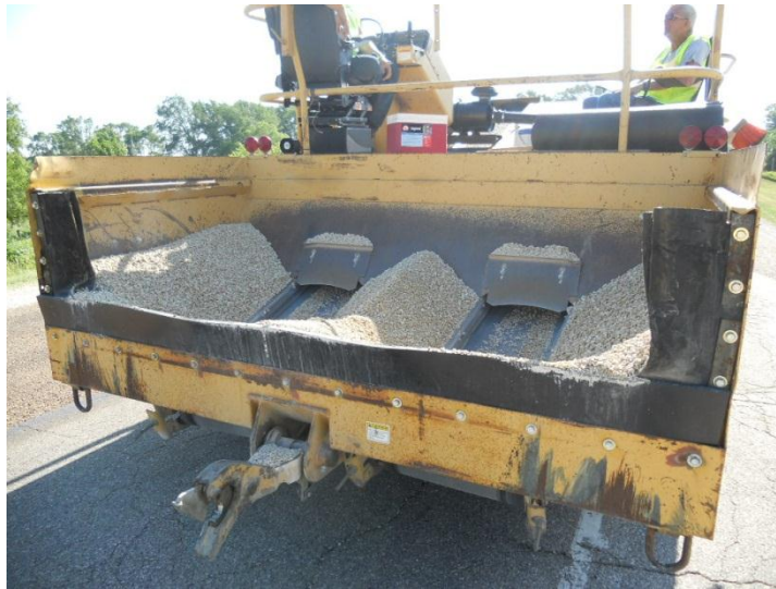
Figure 21: Truck Hook-Up Hitch on Chip Spreader (photo taken by author)
